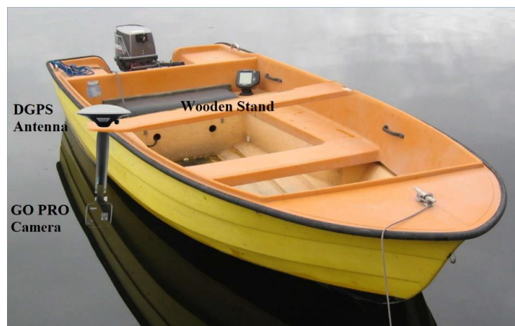
Figure 2. The attached GO PRO camera and differential global positioning system (DGPS) antenna on the motorboat.
